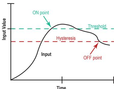
In the example shown, the input is considered on at 15 mA. To consider the input off at 13 mA, set the hysteresis to 2 mA. The input will be considered off when the value is 2 mA less than the threshold.
