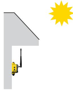
Mount **Vertically** to Avoid **Collecting** Rain. When possible, mount the devices where rain or snow will drain away from the device.
