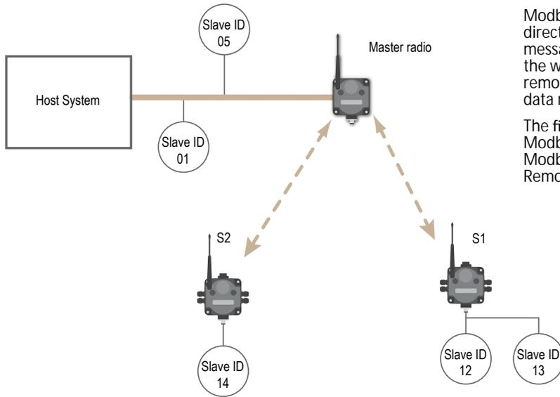
Modbus Slave IDs 01 through 10 are reserved for slaves directly connected to the host (local I/O). As such, polling messages addressed to these devices are not relayed over the wireless link. Use Modbus Slaves IDs 11 through 60 for remote Modbus slaves — devices serially connected to a data radio — allowing a maximum of 50 attached devices.
