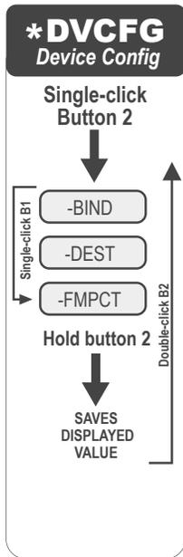
Normally, all devices are bound together before they are physically installed. In a replacement situation, the master device may not always be accessible. Using the manual binding process eliminates the need to put the master device into binding mode and allows the wireless network to remain operational.
