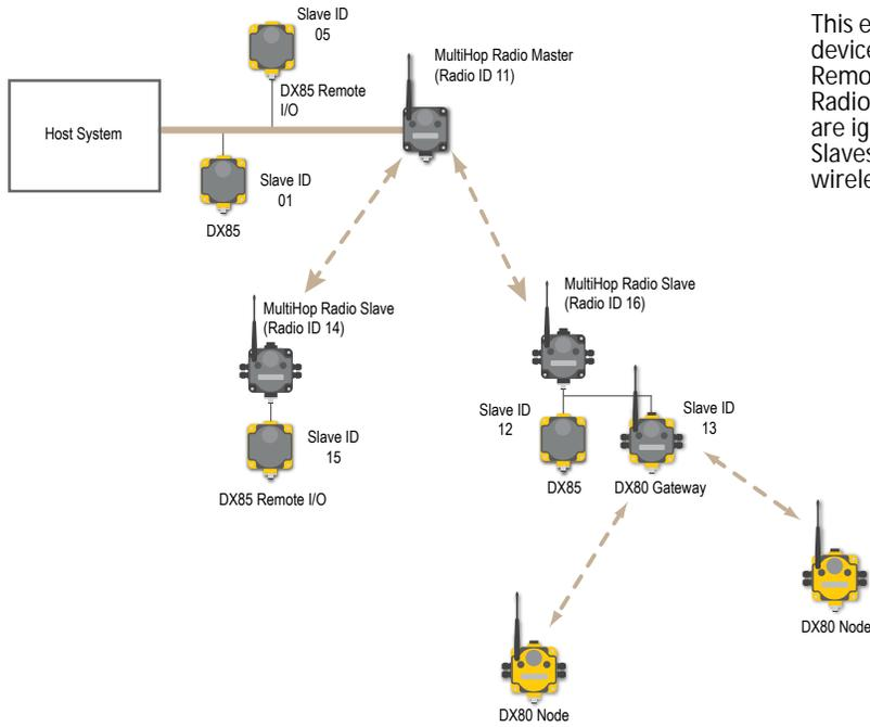
This example host system is connected to three hardwired devices: DX85 Remote I/O Modbus slave 01, DX85 Remote I/O Modbus slave 05, and the master MultiHop Radio. Host messages for Modbus slaves 01 through 10 are ignored by the master radio. Messages for Modbus Slaves or MultiHop Radios 11 through 60 are sent out the wireless network.
