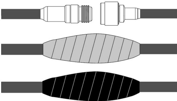
Step 1: Verify both connections are clean and dry before connecting the antenna cable to the antenna or other cable. Hand-tighten the cable connections.
