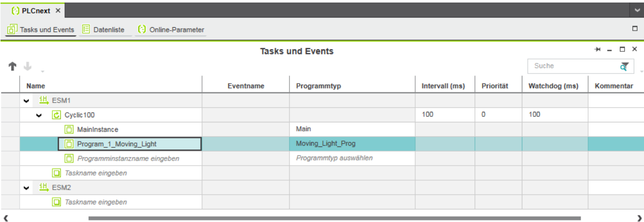
Figure 2-7 Example: tasks and program instances in PLCnext Engineer
