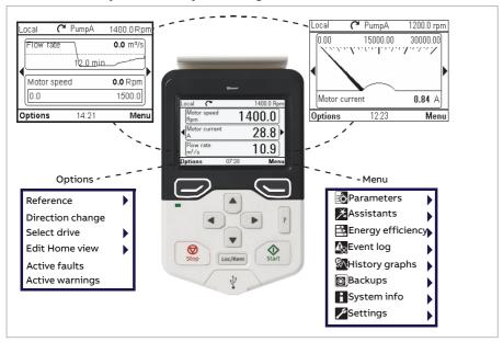
**Note:** The menu shown is an example only. The Menu varies based on the drive/device to which the control panel is connected.
