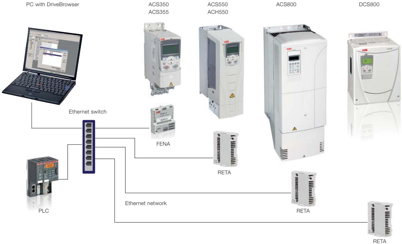
PC connected to drives using the same Ethernet network as the PLC.
