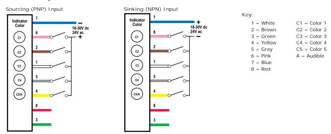
Pin 4 can activate the corresponding color or the audible function, if available. Pins 3 and 8 are not used.
