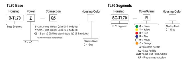
Select the 5-pin/wire base for tower light configurations of up to 4 modules. Select the 7-wire base for tower light configurations of up to 6 modules.
