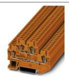
Double-level spring-cage terminal block, connection method: Spring-cage connection, cross section:  $0.08~\text{mm}^2$  -  $4~\text{mm}^2$ , AWG: 28 - 12, width: 5.2~mm, color: orange, mounting type: NS 35/7.5, NS 35/15
