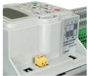
The DG1 drives have an integrated STO function to ensure safe shutdown in case of emergencies. To ensure easy identification of the STO terminals, they are color-coded in yellow (in line with the applicable safety standards) and are arranged separately from the normal control terminals.
