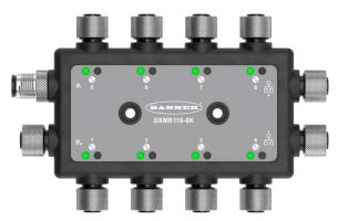
The DXMR110-8K contains eight IO-link ports, allowing for concurrent communication to up to eight IO-Link devices. Data is collected into the internal logic controller to facilitate edge processing, protocol conversion to Industrial Ethernet, Modbus/TCP, and PROFINET, and pushing information to web servers. In addition to IO-Link devices, the IO-Link master can be used to transmit up to 16 discrete signals using pin 2 or pin 4 of the IO-link master ports.
