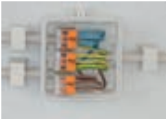
Wiring fine-stranded conductors in junction boxes. Custom low-voltage lighting system Lighting distribution in a ceiling canopy Pendant light connection in a suspended ceiling
