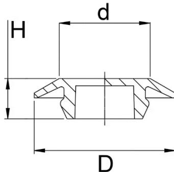
**Sheet Metal Plug - Compatible Hole Diameter 28.6 mm | 1.125 in; Compatible Panel Thickness Range 2.8 mm | 0.110 in; Black**
