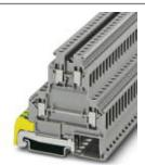
Double-level terminal block, Cross section: 0.2 mm² - 4 mm², AWG: 24 - 10, Connection type: Screw connection, Width: 6.2 mm, Color: gray, Mounting type: NS 35/7,5, NS 35/15
