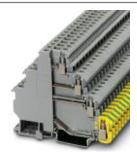
Motor terminal block, four-level, cross section: 0.2 mm² - 4 mm², AWG: 24 - 12, connection method: screw connection, width: 6.2 mm, color: gray, mounting type: NS 35/7,5, NS 35/15
