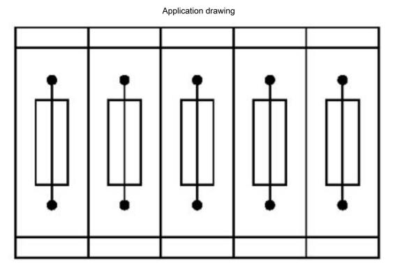
Fuse terminal blocks in interconnected arrangement, block consisting of 5 fuse terminal blocks
