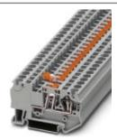
Knife disconnect terminal block, Connection type: Spring-cage connection, Cross section: 0.08 mm² - 6 mm², AWG: 28 - 10, Nominal current: 20 A, Nominal voltage: 400 V, Length: 61.5 mm, Width: 6.2 mm, Color: gray, Assembly: NS 35/7,5, NS 35/15
