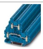
Double-level terminal block, Cross section: 0.14 mm² - 4 mm², AWG: 26 - 12, Connection type: Screw connection, Width: 5.2 mm, Color: blue, Mounting type: NS 35/7,5, NS 35/15
