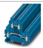
Double-level terminal block with a screw connection, cross section: 0.14 mm² - 6 mm², AWG: 26 - 10, width: 6.2 mm, color: blue
