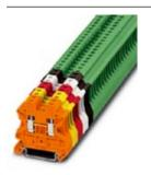
Feed-through terminal block, Connection method: Screw connection, Cross section: 0.14 mm² - 6 mm², AWG: 26 - 10, Width: 6.2 mm, Color: yellow, Mounting type: NS 35/7,5, NS 35/15
