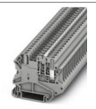
Knife disconnect terminal block, with actuation latch, white disconnect knife, and test socket screws for insertion of test plugs, Connection type: Screw connection, Cross section: 0.14 mm<sup>2</sup> - 6 mm<sup>2</sup>, AWG: 26 - 10, Nominal current: 20 A, Nominal voltage: 500 V, Length: 57.8 mm, Width: 6.2 mm, Color: gray, Assembly: NS 35/7,5, NS 35/15
