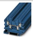
Four-conductor universal terminal block, Connection method: Screw connection, Cross section: 0.14 mm² - 6 mm², AWG: 26 - 10, Width: 6.2 mm, Color: gray, Mounting type: NS 35/7,5, NS 35/15
