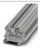
Component terminal block, with integrated diode, Connection method: Screw connection, Cross section: 0.14 mm² - 4 mm², AWG: 26 - 12, Width: 5.2 mm, Color: gray, Mounting type: NS 35/7,5, NS 35/15
