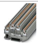
Double-level terminal block, Cross section: 0.14 mm² - 1.5 mm², AWG: 26 - 14, Connection type: Push-in connection, Width: 3.5 mm, Color: gray, Mounting type: NS 35/7,5, NS 35/15
