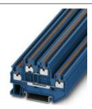
Double-level terminal block, Cross section: 0.14 mm² - 1.5 mm², AWG: 26 - 14, Connection type: Push-in connection, Width: 3.5 mm, Color: blue, Mounting type: NS 35/7,5, NS 35/15
