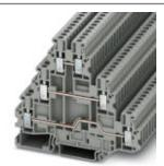
Multi-level terminal block, Cross section: 0.14 mm² - 4 mm², AWG: 26 - 12, Connection type: Screw connection, Width: 5.2 mm, Color: gray, Mounting type: NS 35/7,5, NS 35/15
