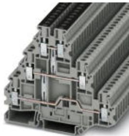
Multi-level terminal block, With equipotential bonder, Cross section: 0.14 mm 2 - 4 mm 2 , AWG: 26 - 12, Connection type: Screw connection, Width: 5.2 mm, Color: gray, Mounting type: NS 35/7,5, NS 35/15
