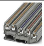
Sensor/actuator terminal block, Connection method: Push-in connection, Cross section: 0.14 mm<sup>2</sup> - 1.5 mm<sup>2</sup>, AWG: 26 - 14, Width: 3.5 mm, Color: gray, Mounting type: NS 35/7,5, NS 35/15
