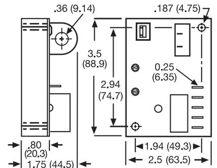
ECS; ECSW (ECS has spade connectors and ECSW has terminal board)
