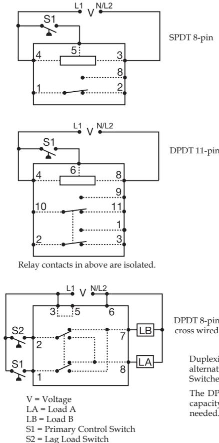
Duplexing (Cross Wired): Duplexing models operate the same as alternating relays and when both the Control (S1) and Lag Load (S2) Switches are closed, Load A and Load B energize simultaneously.
