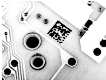
Figure 157. Data Matrix Code Directly Marked on PCB Surface by Using Laser Etching Technology
