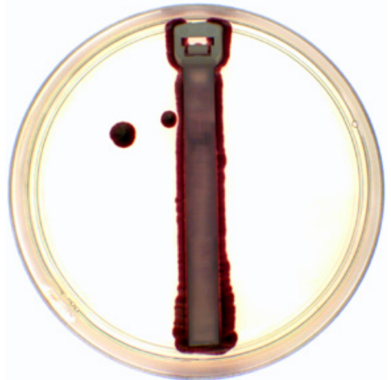
Standard cable tie after 24 hours of exposure to bacteria
