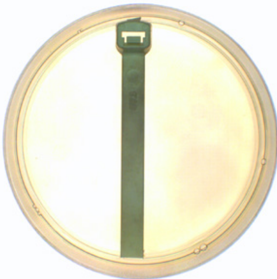
Ty-Fast Ag+ after 24 hours of exposure to bacteria
