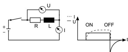
**Switching Relay Coils.**
