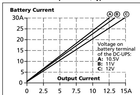
Fig. 6-2 Required input current vs. input voltage for battery charging
