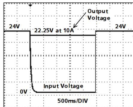
Fig. 5-3 Available output current in buffer mode
