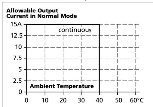
Fig. 16-2 **Buffer Mode: Output current vs. ambient temperature**
