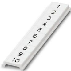
Zack Marker strip, flat, Strip, white, labeled, Printed vertically: consecutive numbers 1 ... 10, 11 ... 20, etc. up to 91 ... 100, mounting type: latching, for terminal block width: 3.5 mm, Number of individual labels: 10, text field height: 5. 15 mm, text field width: 3.5 mm
