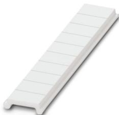
Zack Marker strip, flat, can be ordered: Strip, white, labeled according to customer specifications, mounting type: snap into flat marker groove, for terminal block width: 3.5 mm, Number of individual labels: 10, text field height: 5.2 mm, text field width: 3.5 mm
