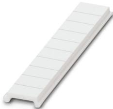
Zack Marker strip, flat, Strip, white, unmarked, can be labeled with: PLOTMARK, CMS-P1-PLOTTER, mounting type: latching, for terminal block width: 3.5 mm, Number of individual labels: 10, text field height: 5.2 mm, text field width: 3.5 mm
