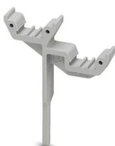
Marker carriers, snaps into the PT 1,5/S-3L Push-in three-level terminal block, can be marked with UCT-TM 3,5, UCT-TMF 3,5, ZB 3,5, or ZBF 3,5, gray, unmarked, mounting type: plug in, text field height: 10.5 mm, text field width: 3.5 mm
