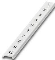
Zack Marker strip, flat, Strip, white, labeled, Printed vertically: consecutive numbers 1 ... 10, 11 ... 20, etc. up to 91 ... 100, mounting type: latching, for terminal block width: 6.2 mm, Number of individual labels: 10, text field height: 6.15 mm, text field width: 5.15 mm
