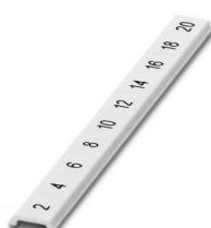
Zack Marker strip, flat, Strip, white, labeled, printed horizontally: consecutive even numbers 2 ... 20, 22 ... 40, etc. up to 82 ... 100, mounting type: latching, for terminal block width: 6.2 mm, Number of individual labels: 10, text field height: 6.15 mm, text field width: 5.15 mm
