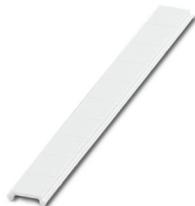
Zack Marker strip, flat, Strip, can be ordered: Strip, white, labeled according to customer specifications, mounting type: snap into flat marker groove, for terminal block width: 6.2 mm, Number of individual labels: 10, text field height: 6.15 mm, text field width: 5.15 mm
