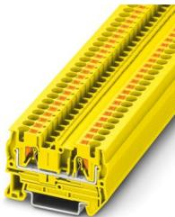
Feed-through terminal block, nom. voltage: 800 V, nominal current: 32 A, number of connections: 2, connection method: Push-in connection, Rated cross section: 4 mm<sup>2</sup>, cross section: 0.2 mm<sup>2</sup> - 6 mm<sup>2</sup>, mounting type: NS 35/7,5, NS 35/15, color: yellow
