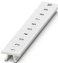
Zack marker strip, Strip, white, labeled, can be labeled with: CMS-P1-PLOTTER, printed horizontally: consecutive numbers 1 ... 10, 11 ... 20, etc. up to 491 ... 500, mounting type: latching, for terminal block width: 6.2 mm, Number of individual labels: 10, text field height: 10.5 mm, text field width: 6.15 mm
