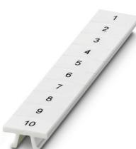
Zack marker strip, Strip, white, labeled, can be labeled with: CMS-P1-PLOTTER, Printed vertically: consecutive numbers 1 ... 10, 11 ... 20, etc. up to 491 ... 500, mounting type: latching, for terminal block width: 6.2 mm, Number of individual labels: 10, text field height: 10.5 mm, text field width: 6.15 mm
