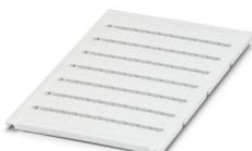
Marker for terminal blocks, Sheet, white, unmarked, can be labeled with: BLUEMARK E.CARD, BLUEMARK ID COLOR, BLUEMARK ID, BLUEMARK CLED, PLOTMARK, CMS-P1-PLOTTER, mounting type: latching, for terminal block width: 6.2 mm, Number of individual labels: 80, text field height: 10.5 mm, text field width: 5.6 mm
