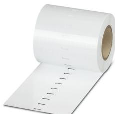
Marker for terminal blocks, Roll, white, unmarked, can be labeled with: THERMOMARK ROLL 2.0, THERMOMARK ROLL, THERMOMARK ROLL X1, THERMOMARK ROLLMASTER 300/600, THERMOMARK X1.2, THERMOMARK S1.1, perforated, mounting type: latching, snap into flat marker groove, for terminal block width: 6.2 mm, Number of individual labels: 16000, text field height: 6.35 mm, text field width: 6.15 mm
