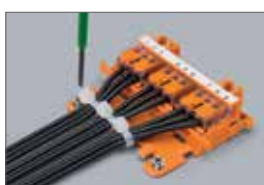
Horizontal mounting with strain relief plate on flat panel; wiring locations identified using marker strips
