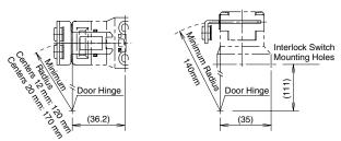
When the door hinge is on the extension line of the actuator mounting surface:
