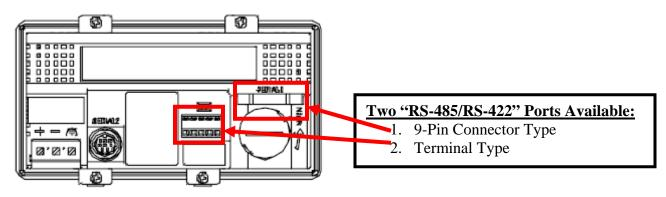
Part Number <u>HG1F-SB22YF-\*</u>, has two available RS- 485/RS- 422 ports to communicate with the PLC (use either 9- Pin Connector or Terminal Type).
