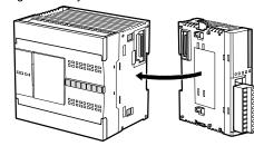
Note: I/O modules cannot be mounted on FC5A-C10R2, -C10R2C, -C10R2D, -C16R2, -C16R2C, -C16R2D and -C24R2D\*
