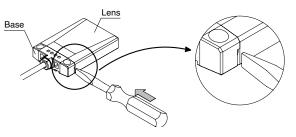
2. Twist the screwdriver and disengage the lens from the base.
