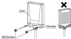
Note 1: Do not install the LH indicator by attaching the lens only, such as by taping down on the lens as the internal components may come loose.
