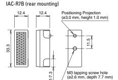
Material: PMMA (reflector), ABS (base)
