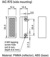
Material: PMMA (reflector), ABS (base)
