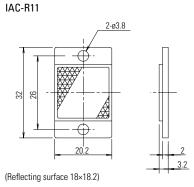
Material: PMMA (reflector), ABS (base)
