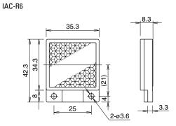
(Effective reflecting area: 30 × 31) Material: PMMA (reflector), ABS (base)
