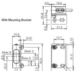
Note 1: Projector (through-beam)Receiver (through-beam) Note 2: Projector (polarized retroreflective, background suppression) Note 3: Receiver (polarized retroreflective)
