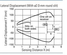
SA1E-T -NA (Infrared LED w/o sensitivity adjustment) 1-2. Through-beam
