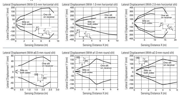
2-1. Polarized Retroreflective SA1E-P (Red LED w/sensitivity adjustment)
