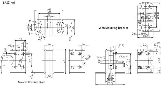
Note 1: Projector (through-beam)Receiver (through-beam) Note 2: Projector (polarized retroreflective, background suppression) Note 3: Receiver (polarized retroreflective)
