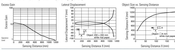
4. Small-beam Reflective SA1E-N (Red LED w/sensitivity adjustment)
