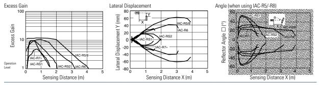
2-2. Polarized Retroreflective SA1E-P□-NA (Red LED w/o sensitivity adjustment)
