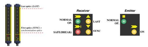
Signals are clearly identified through symbols allowing immediate reading, independent of bars directions. A short description of the signalling LEDs is necessary to avoid misunderstandings.
