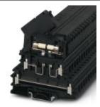
Fuse modular terminal block, Connection method: Screw connection, Cross section: 0.2 mm²- 4 mm², AWG: 24 - 12, Nominal current: 32 A, Nominal voltage: 400 V, Width: 8.2 mm, Fuse type: G / 6,3 x 32, Fuse type: Glass / ceramics / ..., Mounting type: NS 35/7,5, NS 35/15, NS 32, Color: black
