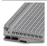
Potential distributors, Nom. voltage: 500 V, Nominal current: 24 A, Cross section: 0.14 mm² - 4 mm², AWG: 12 - 26, Connection type: Spring-cage connection, Number of connections: 2, Width: 5.2 mm, Length: 141 mm, Color: gray, Assembly: NS 35/7,5, NS 35/15
