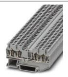
Feed-through terminal block, Connection method: Spring-cage connection, Cross section: 0.08 mm² - 4 mm², AWG: 28 - 12, Width: 5.2 mm, Color: red, Mounting type: NS 35/7,5, NS 35/15
